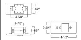
Face Width: 4-1/2" Housing Width: 3-5/8" Face Length: 2-3/4" Housing Length: 1-1/2" Housing Depth: 1-1/8"
