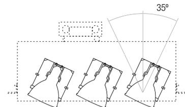
**PAR30 Lamp Holder for Trimless Multiple Lighting Housings - Requires NMRTL Housing**
