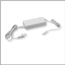
Direct Plug-In LED Driver NATL-596W 24V 96W Input Voltage: 120V Input Wire: 44" Cord and Plug Output Wire: 58" Power line connector
