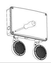
Remove screws to open the front cover.
