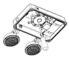
Knock out center and appropriate mounting screw holes on the back plate.
