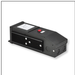
Class 2 Hardwire LED Driver with Regulator, MLV Dimming NMTD-60/24D 24V 60W NMTD-96/24D 24V 96W Input Voltage: 120-277V Dimming: Magnetic Low Voltage Regulator: Integral regulator for constant current and voltage Includes: 10' Power Line Connector
