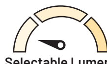
Selectable Lumens Three position sliding switch 7000lm / 7500lm / 8000lm
